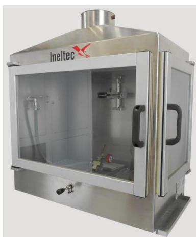
**PHOTO 12 : EQUIPEMENT POUR REALISER LES ESSAIS D'INFLAMMABILITE**
